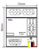
Figure 2. Dimensions - Front View
