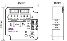
Figure 2. Dimensions-Front View
