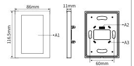
Figure 2. Dimensions - Front View Figure 3. Side View Figure 4. Back View
